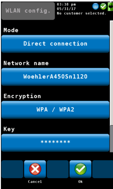
Fig. 33: WLAN configuration – Direct connection
