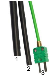
Fig. 16: Gas probe – gas hose (1), pressure hose (2), temperature plug (3)
