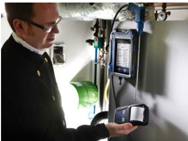
Printing the readings of the Wohler A 450 on the Thermoprinter Wohler TD 100.
