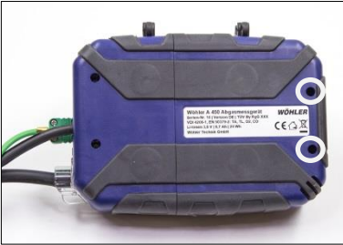
Fig. 48: Bottom of the device - Open the cover by loosening the cross-head screws .
